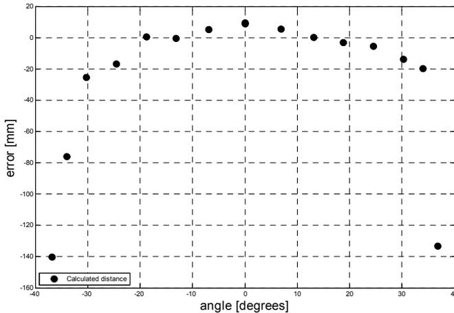
Fig. 7 – Beam pattern of ultrasonic sensors.
