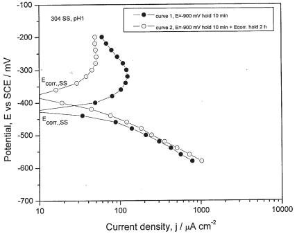
Fig. 5. Two potentiodynamic curves for the same stainless steel electrode after "activation" at -0.900 V (SCE) for 10 min. Curve 1 – starting from the cathodic potential; curve 2 – starting after 2 h hold from  $E_{\text{cor.SS}}$  first in the anodic direction.
