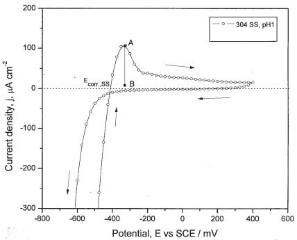
Fig. 3. Cyclic volammogram for the stainless steel electrode after cathodic "activation" at -0.900 V (SCE) for 10 min. Points A and B connect the current decay during hold of the potential.
