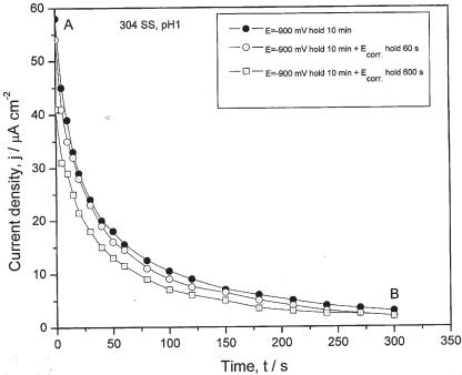
Fig. 4. Depandence of the current over time during hold of potential at the potential corresponding to point A depicted in Fig. 3, but after different holds at the corrosion potential after "activation";  $\bullet$  – immediately after "activation";  $\circ$  – after 600 s.
