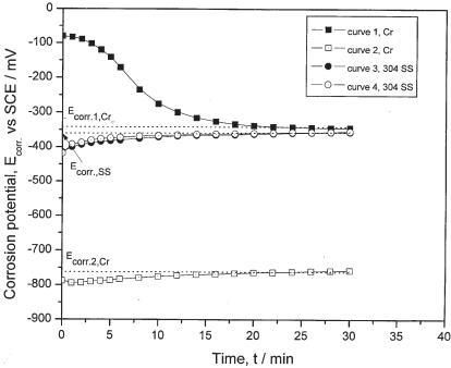
Fig. 1. Change of the open circuit potential over time after introduction of the electrode into the deaerated sulfuric acid (pH 1) (curve 1 for Cr and curve 3 for steel) and after the cathodic "activation" (curve 2 for Cr and 4 for steel). Potentials  $E_{\rm cor.1,Cr}$ , and  $E_{\rm cor.5,S}$  correspond to passive state corrosion potentials for Cr and stainless steel, respectively.  $E_{\rm cor.1,Cr}$  is the corrosion potential of the active chromium.
