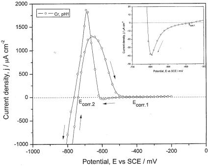
Fig. 2. Cyclic voltammogram for the Cr electrode after cathodic activation. Inset presents the enlarged cathodic peak in the reverse scan, representing cathodic hydrogen evolution on the passive surface
