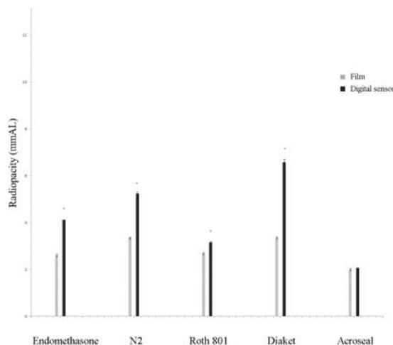
Fig. 3 – Radiopacity of the tested endodontic materials expressed as an equivalent thickness of aluminum. \* – statistically significant difference on the digital sensor related to that on film (paired *t*-test;  $p < 0.05$ ).
