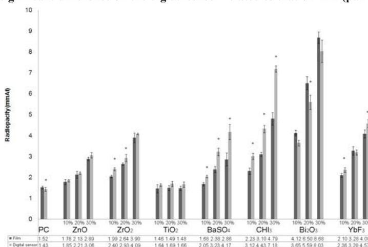
Fig. 4 – The mean radiopacity values and standard deviations expressed in thickness of aluminum (Al) for Portland mixtures. The columns marked with \* represent groups with significantly different radiopacity on digital sensor when compared with film (paired *t*-test;  $p < 0.05$ ).
