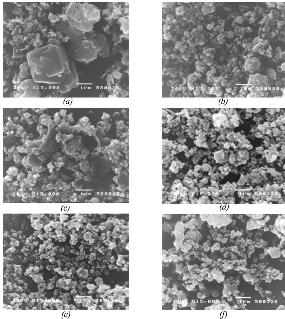
**Fig. 2** SEM micrographs for the ZnO-TiO<sub>2</sub> system 1:1 mechanically activated for different times a) non-activated mixture, b) 5 minutes, c) 10 minutes, d) 20 minutes, e) 80 minutes and f) 160 minutes.
