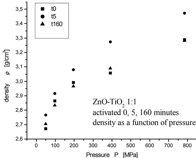
**Fig. 5** Density as a function of pressure in a process of compacting ZnO-TiO<sub>2</sub> powders activated for different times: t0-non-activated mixture (0 minutes), t5-activated 5 minutes and t160-activated 160 minutes.
