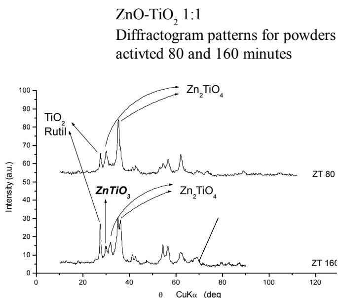
**Fig. 4** XRD profiles of ZnO-TiO<sub>2</sub> powders 1:1 mechanically activated 80 and 160 minutes.
