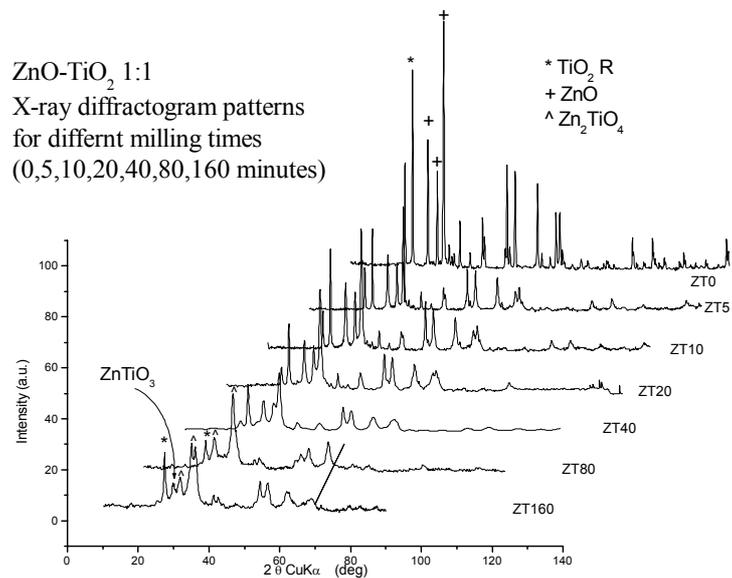
**Fig. 3** XRD profiles of ZnO-TiO<sub>2</sub> powders 1:1 mechanically activated for different times (0, 5, 10, 20, 40, 80 and 160 minutes).
