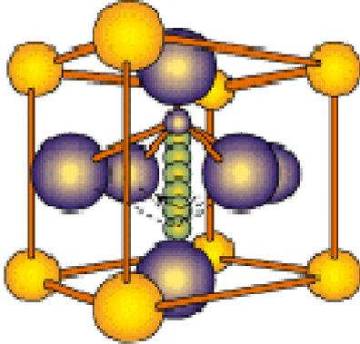
Fig. 4 Ion positions in tetragonal BaTiO<sub>3</sub> [3]
