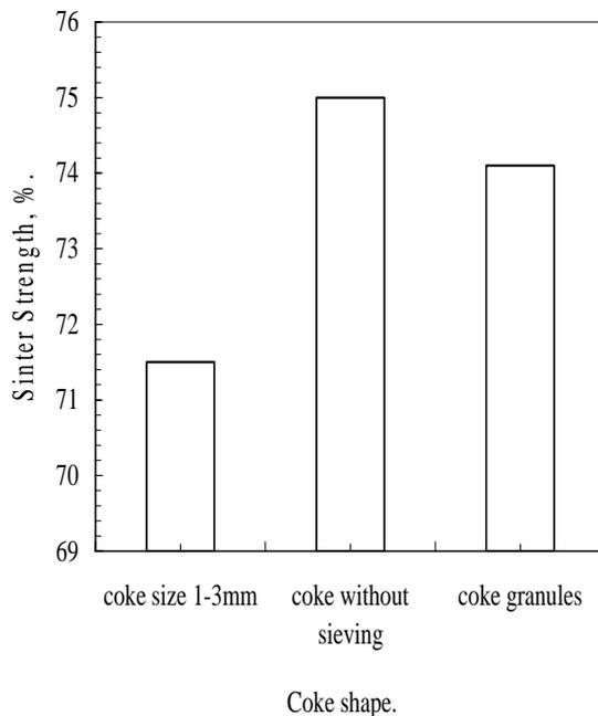
**Fig.5** Effect of coke shape on the strength of produced sinter.
