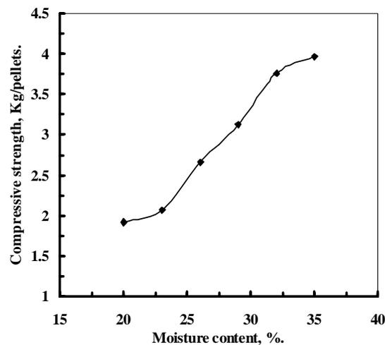
**Fig.3.** Effect of moisture content added on the compressive strength of dried granules.
