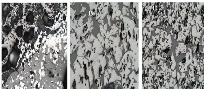
**Fig.9** Microscopic structure of produced sinter by using different coke breeze shapes, (A = coke breeze -3+1 mm, B = coke breeze without sieving, C = coke breeze granules.)
