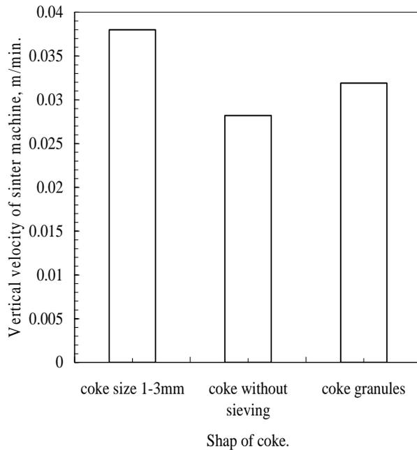
**Fig.4** Effect of coke shape on the vertical velocity of sinter machine
