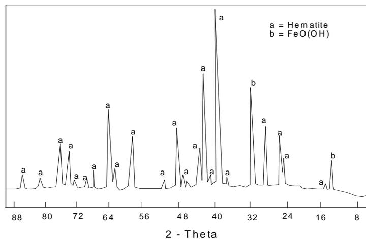
**Fig.1.** X-ray diffraction of iron ore.
