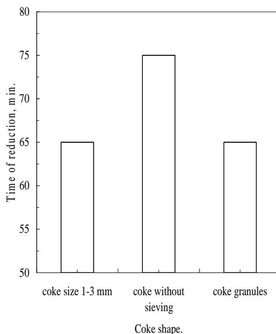
**Fig.8** Effect of coke shape on the reduction time of produced sinter.
