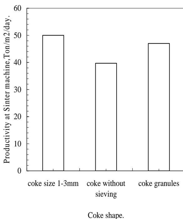
**Fig.6** Effect of coke shape on the productivity of sinter machine.
