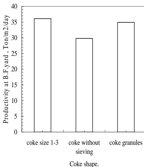
**Fig.7** Effect of coke shape on the productivity of blast furnace.
