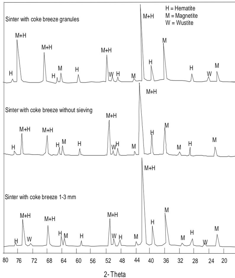
**Fig. 10.** X-ray diffraction of iron ore sinter by using different shape of coke breeze
