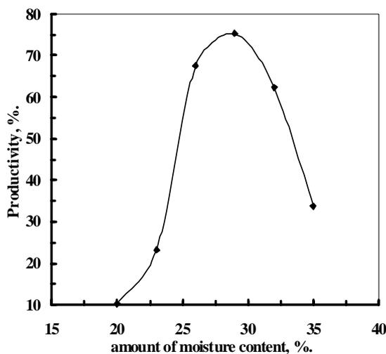
**Fig 2.** The effect of moisture content on the productivity of green granules ( Moisture content =.amount of molasses + 10 % water)
