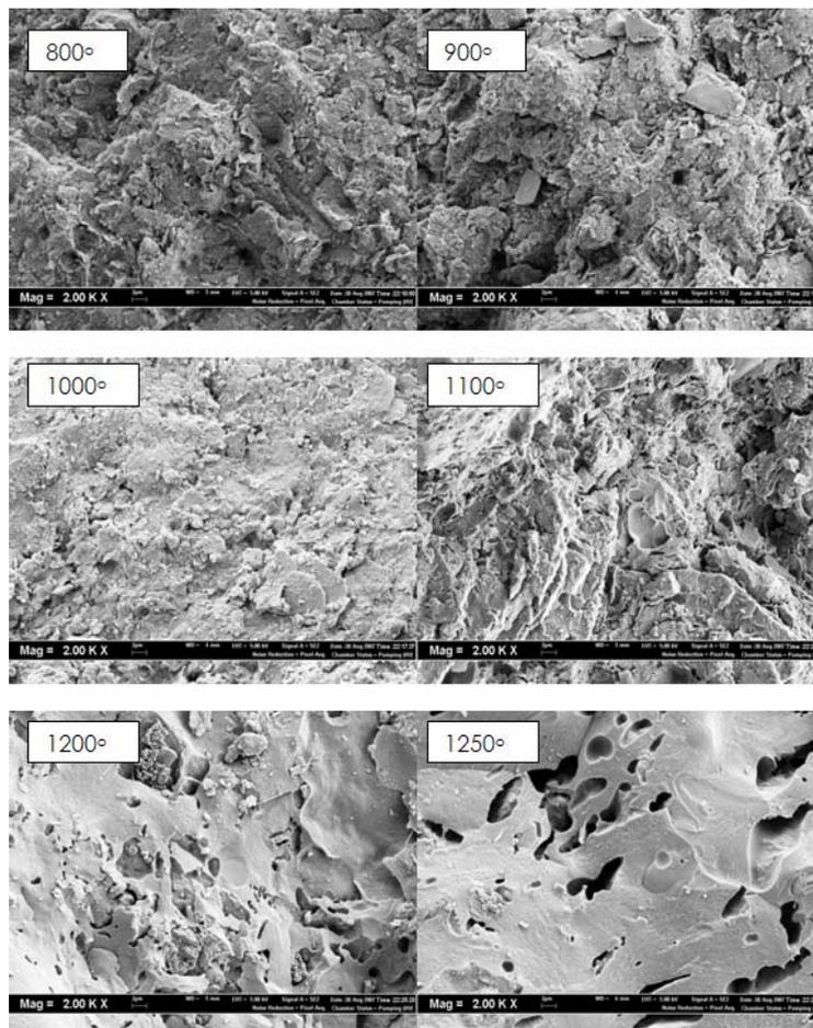
**Fig. 6.** SEM micrographs for the clay fired at different temperatures
