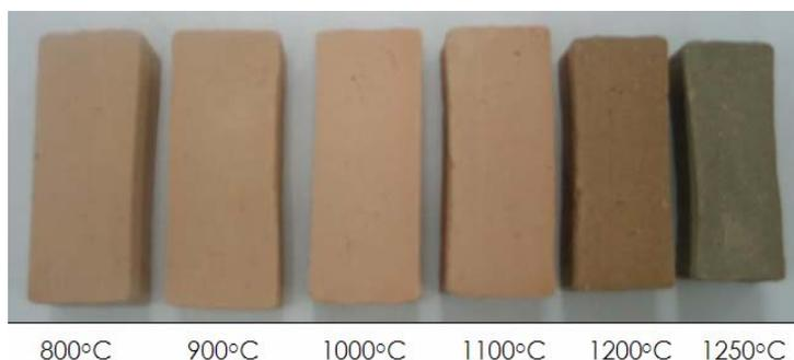
Fig 3. Effect of firing temperature on the colour and shrinkage of the clay
