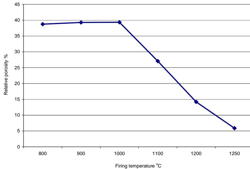
**Fig. 7.** Effect of firing temperature of the clay on the porosity
