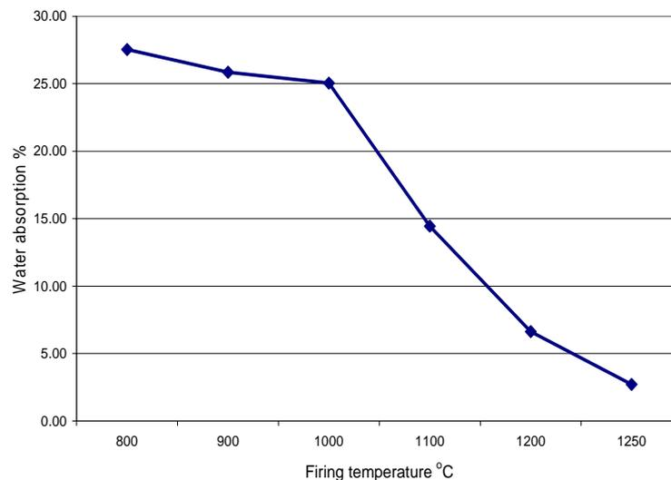
**Fig. 8.** Effect of firing temperature of the clay on the water absorption
