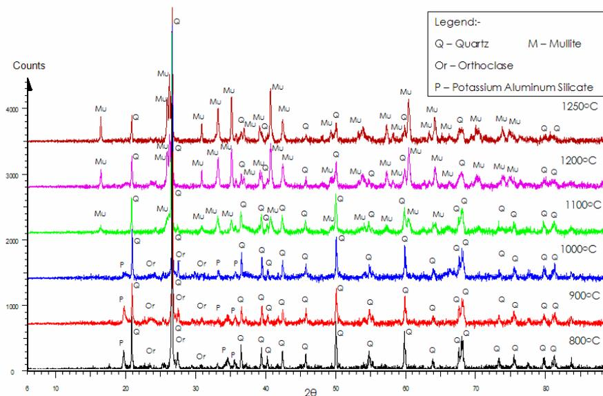
Fig. 5. XRD diffractograms of the clay fired at different temperatures
