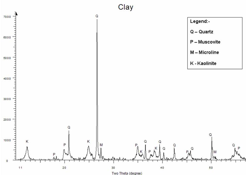
**Fig. 2.** XRD diffractogram of clay taken from Beruas, Malaysia
