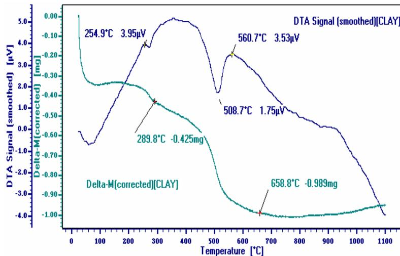
Fig. 4. Thermogravimetric and differential thermal analyses of the raw clay
