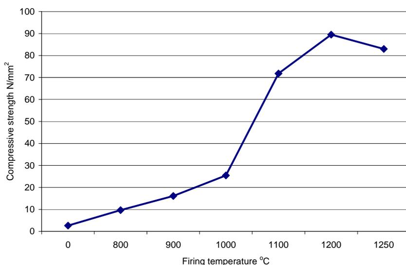
**Fig. 9.** Effect of firing temperature of the clay on the compressive strength
