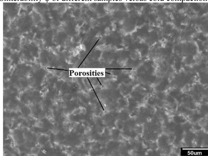
Fig. 9. SEM image of WC sintered samples.
