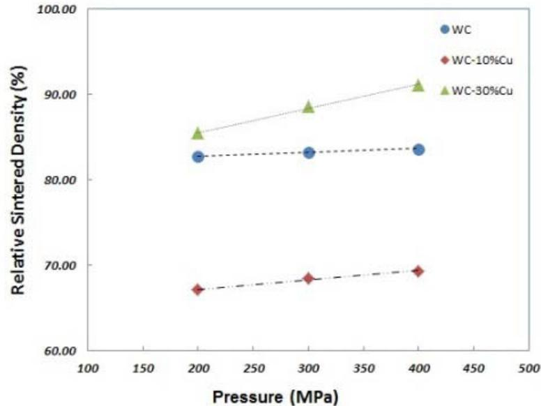
**Fig. 7.** The effect of cold compaction pressure magnitude on the relative density of the sintered samples at 1400°C.
