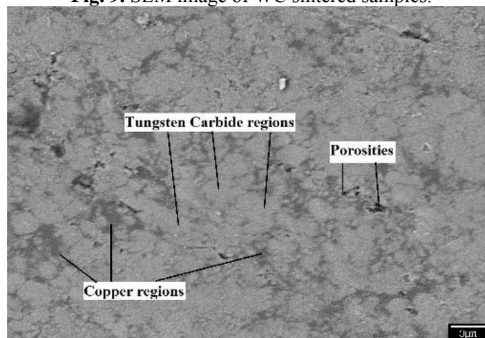
Fig. 10. SEM image of WC/Cu composites. The white, gray and black regions are tungsten carbide, copper and porosity regions, respectively.
