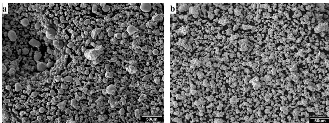
**Fig.1.** SEM image of the as received powders (a) Copper (b) Tungsten Carbide.
