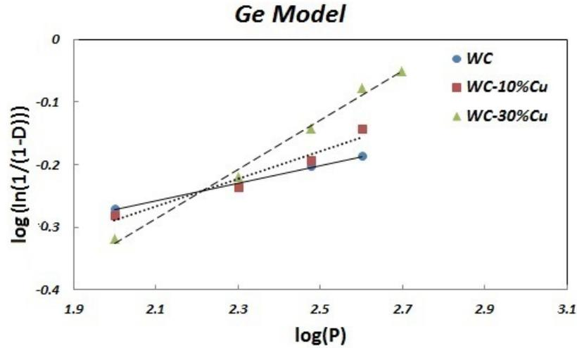
**Fig. 6.**  $\log\left(\ln\left(\frac{1}{1-D}\right)\right)$  versus uniaxial pressure compaction magnitude  $\log(P)$  for different samples (The Ge equation).
