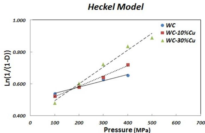
**Fig. 4.**  $\ln\left(\frac{1}{1-D}\right)$  versus uniaxial pressure compaction magnitude (P) for different samples (The Heckel equation).
