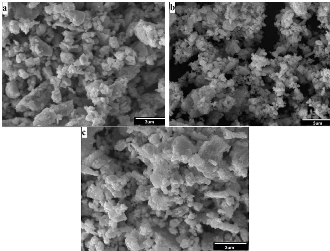
**Fig. 2** SEM image of the as milled powders (a) WC (b) WC-10%wtCu (c) WC-30%wtCu
