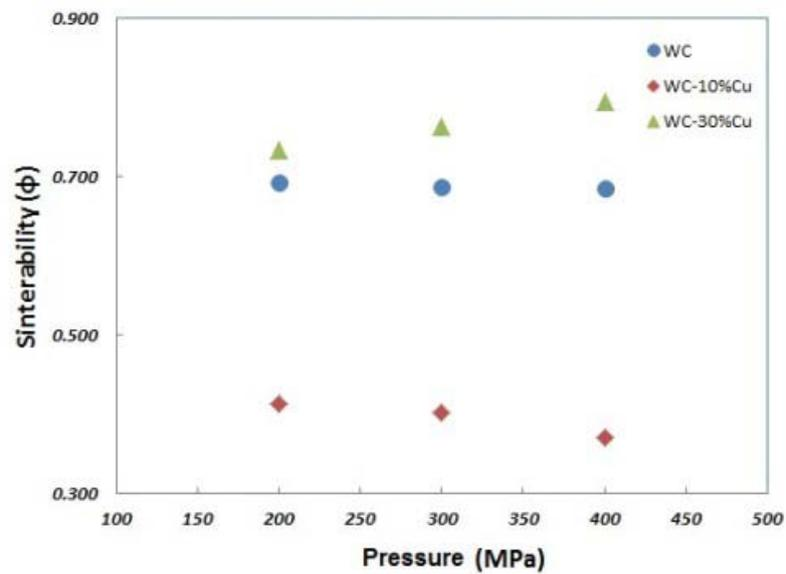
Fig. 8. Sinterability  $\phi$  of different samples versus cold compaction pressure.
