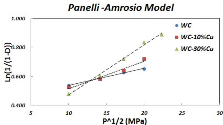
**Fig. 5.**  $\ln\left(\frac{1}{1-D}\right)$  versus the square root of uniaxial pressure compaction magnitude  $P^{1/2}$  for different samples (The Panelli-Ambrosio equation).
