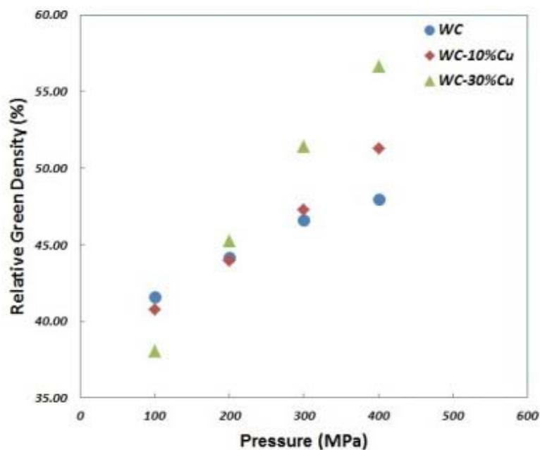
**Fig. 3.** The effect of cold compaction pressure on the relative green density for different samples.
