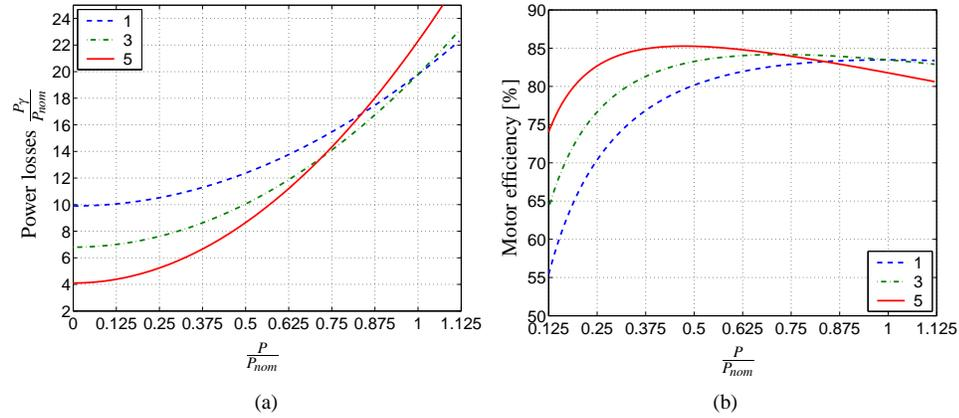
Fig. 1. (a) The total losses versus  $P_\gamma/P_n = f(P/P_n)$ , and (b) Efficiency curve  $\eta = f(P/P_n)$ , in relation to three  $P_0/P_\gamma$  values (in a per unit  $P_n = 1$ ):  $P_0/P_\gamma = 0.099/0.099$ ,  $\eta_{max} = \eta_n$  (for  $P = P_n = 100\%$ ) curve 1 - motor 1,  $P_0/P_\gamma = 0.068/0.130$ ,  $\eta_{max} = \eta_{75}$  (for  $P/P_n = 75\%$ ), curve 3- motor 2,  $P_0/P_\gamma = 0.041/0.182$ ,  $\eta_{max} = \eta_{50}$  (for  $P/P_n = 50\%$ ), curve 5-motor 3.
