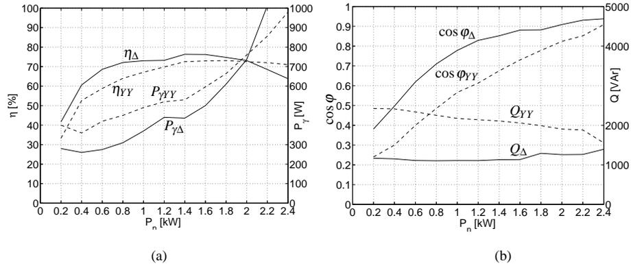
Fig. 3. (a) Efficiency ( $\eta$ ) and power losses ( $P_\gamma$ ), and (b) Factor power ( $\cos \phi$ ) and reactive load ( $Q$ ) versus power output ( $P$ ), for rewinding motor 1ZK 100 L-4, 2.2 kW: For winding in "YY" connection (corresponding to nominal voltage  $U_n$ ), and For winding in "Δ" connection (corresponding to voltage value  $0.866U_n$ ).
