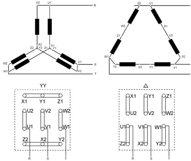
Fig. 2. Induction motors with YY/ $\Delta$  connection change for efficiency and power factor increasing at partial loads
