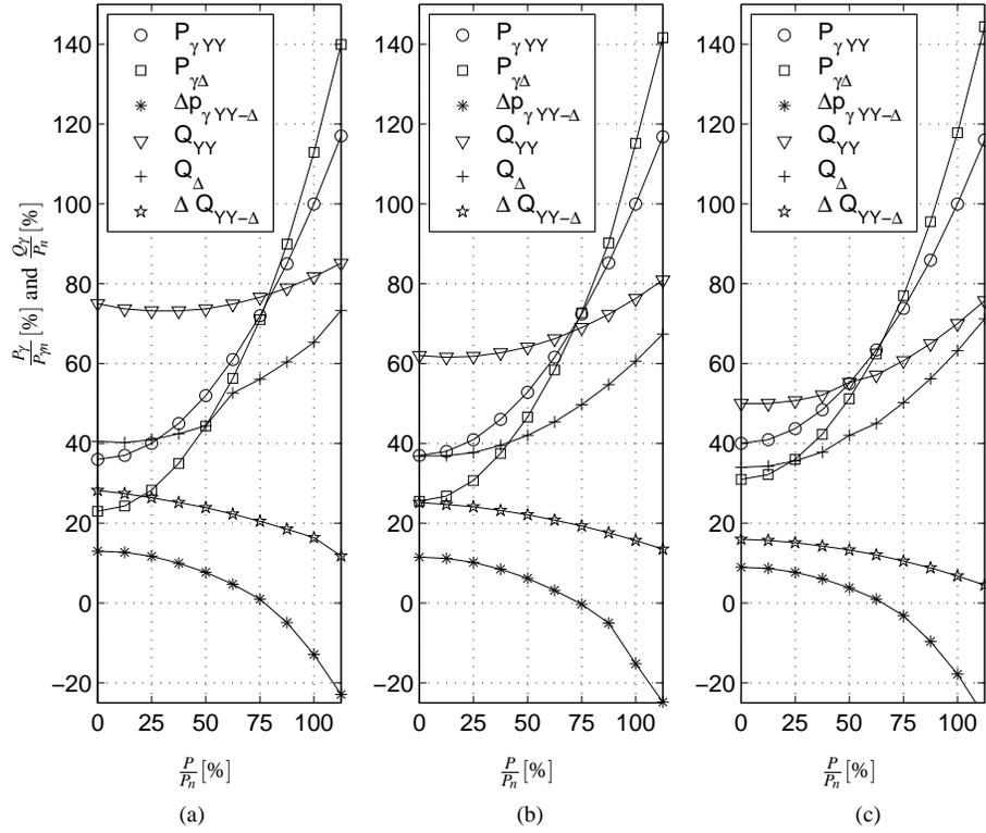
Fig. 4. Dependencies of total losses ( $P_{\gamma}\% = P_{\gamma}/P_{\gamma,n}\%$ ) and reactive loads ( $Q\% = Q/Q_n\%$ ), as a corresponding changes of total losses  $\Delta P_{\gamma YY-\Delta}\% = P_{\gamma YY} - P_{\gamma\Delta}\%$  and reactive loads  $\Delta Q_{YY-\Delta}\% = Q_{YY} - Q_{\Delta}\%$ , with YY/ $\Delta$  connection change, for motors (a) small, (b) medium and (c) greater power.
