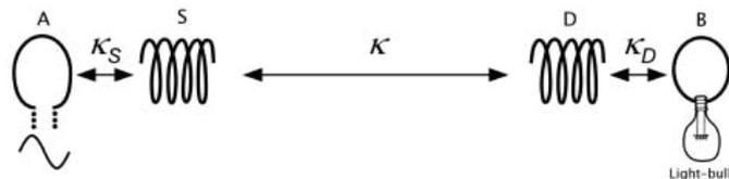
**Fig. 4** Simplified schematic diagram of magnetic resonant energy transfer: driver coil A, resonant source S, receiver device resonant coil D, and the bulb (load) B coil
