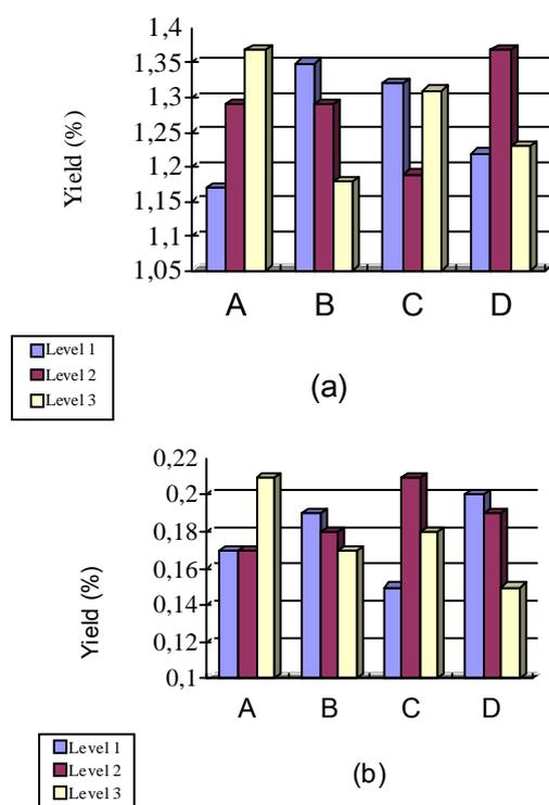
**Fig. 4.** The yields of GPA (a) and GPS (b) by EE under orthogonal conditions (for designations of factors A, Extraction temperature (35, 40, 45 °C); B, pH value of solvent (5.0, 6.0, 7.0); C, Solid-enzyme ratio (1000:1, 1000:2, 1000:3), and D, Extraction time (0.5, 1.0, 1.5 h).
