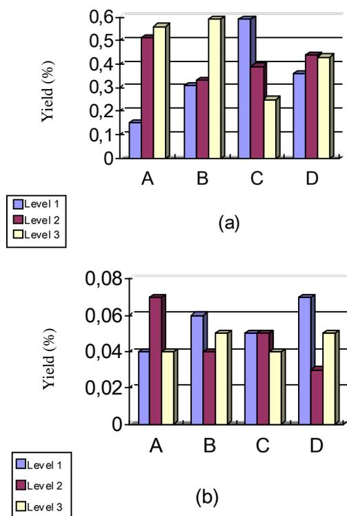
**Fig. 3.** The yields of GPA (a) and GPS (b) by SFE under orthogonal conditions (for designations of factors A, Temperature (40, 50, 60 °C); B, time (2.0, 3.0, 4.0 h); C, flow rate (15, 20, 25 L/h), and D, Modifier volume (200, 300, 400 ml).
