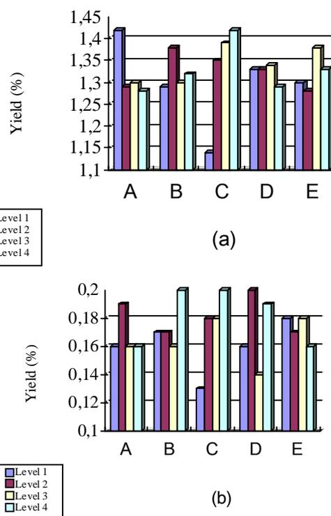
**Fig. 2.** The yields of GPA (a) and GPS (b) by SE under orthogonal conditions (A, extraction temperature (50, 60, 70, 80 °C); B, extraction time (0.5, 1.0, 1.5, 2.0 h); C, extraction times (1, 2, 3, 4); D, ethanol concentration (50%, 60%, 70%, 80%), and E, Solvent volume (10, 12, 14, 16 ml/g).
