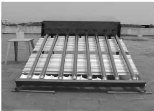
Figure 3. Pictorial view of solar still augmented with evacuated tubes
