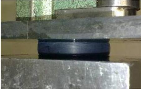
**Figure 4.** A rubber sample in a compressed state at true strain value of  $-1.1$
