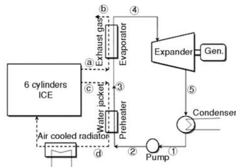
Figure 1. Preheat configuration combined with the ICE
