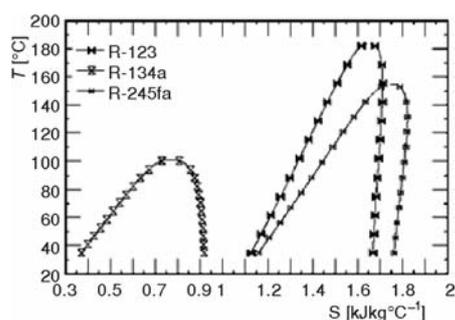
Figure 3. *T-s* diagram for considered working fluids
