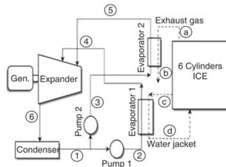
Figure 2. Two-stage configuration combined with the ICE
