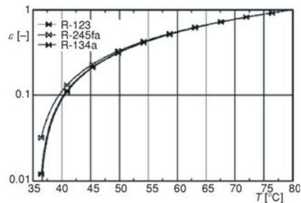
**Figure 18. Preheater effectiveness vs. temperature**
