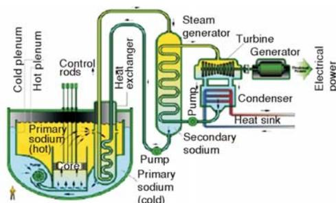
Figure 5. FBR with closed fuel cycle
