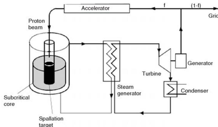
**Figure 7. Accelerator driven system – ADS**
