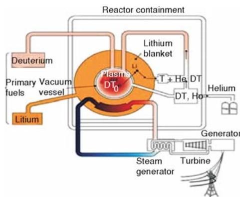
Figure 6. Fusion power plant
