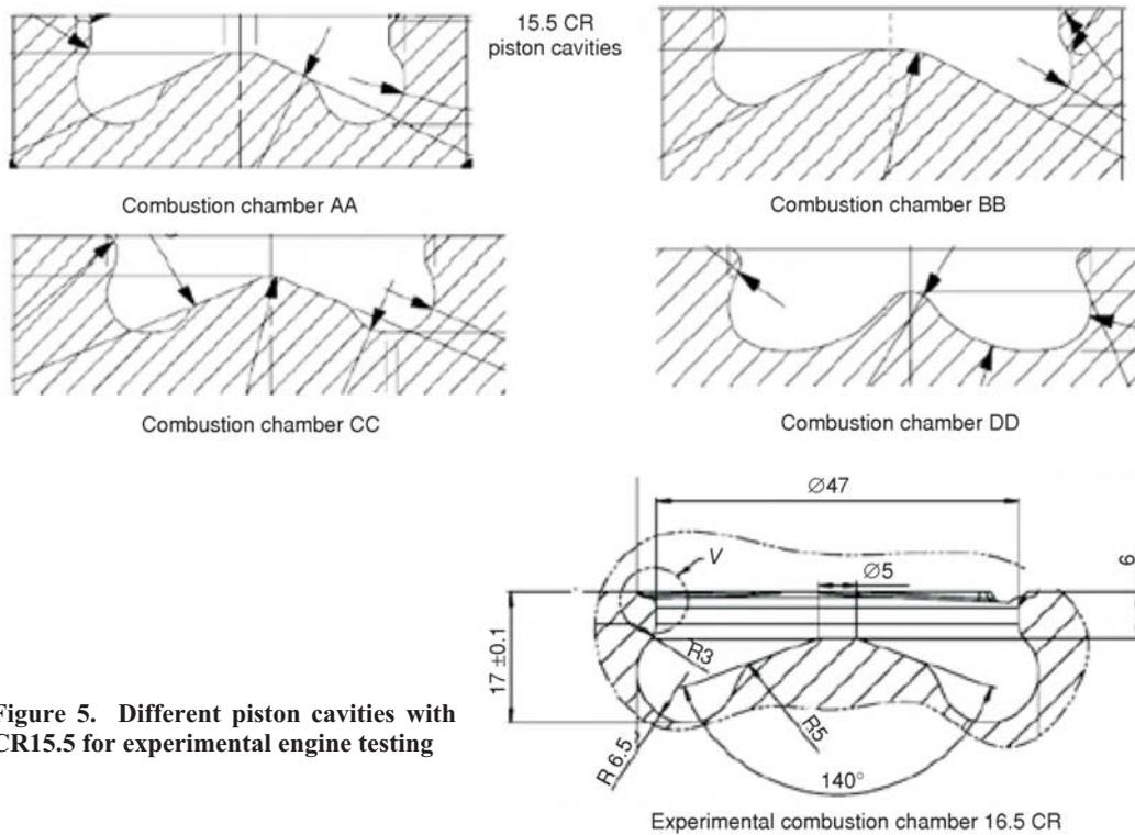
Figure 5. Different piston cavities with CR15.5 for experimental engine testing
