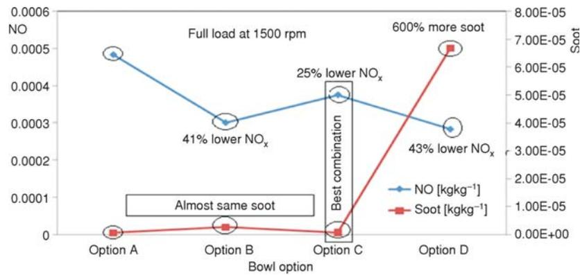
Figure 7. Cumulative NO comparisons and soot of different combustion chambers at 1500 rpm full load point
