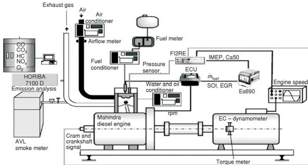
Figure 6. Schematic of experiment set-up with measurement system
