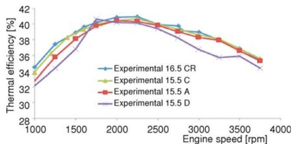
Figure 11. Comparison of brake thermal efficiency of engine with different combustion chambers at full load performance
