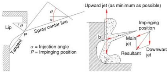
Figure 3. Fuel spray jet hitting direction and movement
