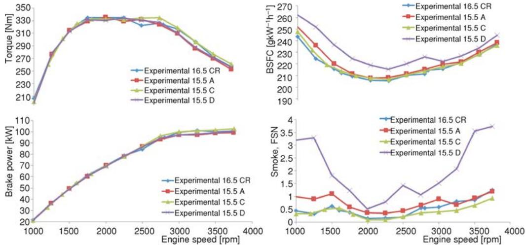
Figure 10. Full load performance comparison of engine with different combustion chambers
