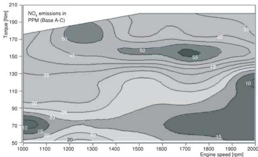
Figure 9.  $\text{NO}_x$  emission (PPM) difference with combustion chamber A and C
