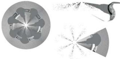
Figure 4. Injector holes and swirl matching through CFD analysis
