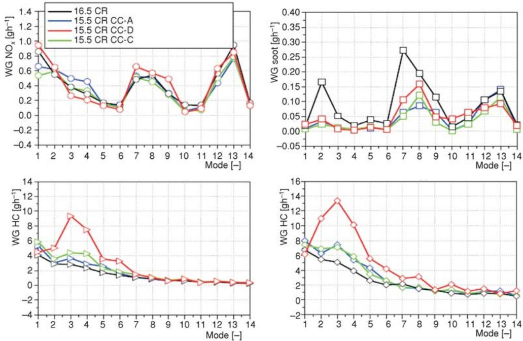
Figure 12. 14 mode emission comparison of engine with different combustion chambers (for color image journal web site)
