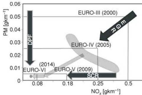
**Figure 1. European emission regulations for passenger cars application**
