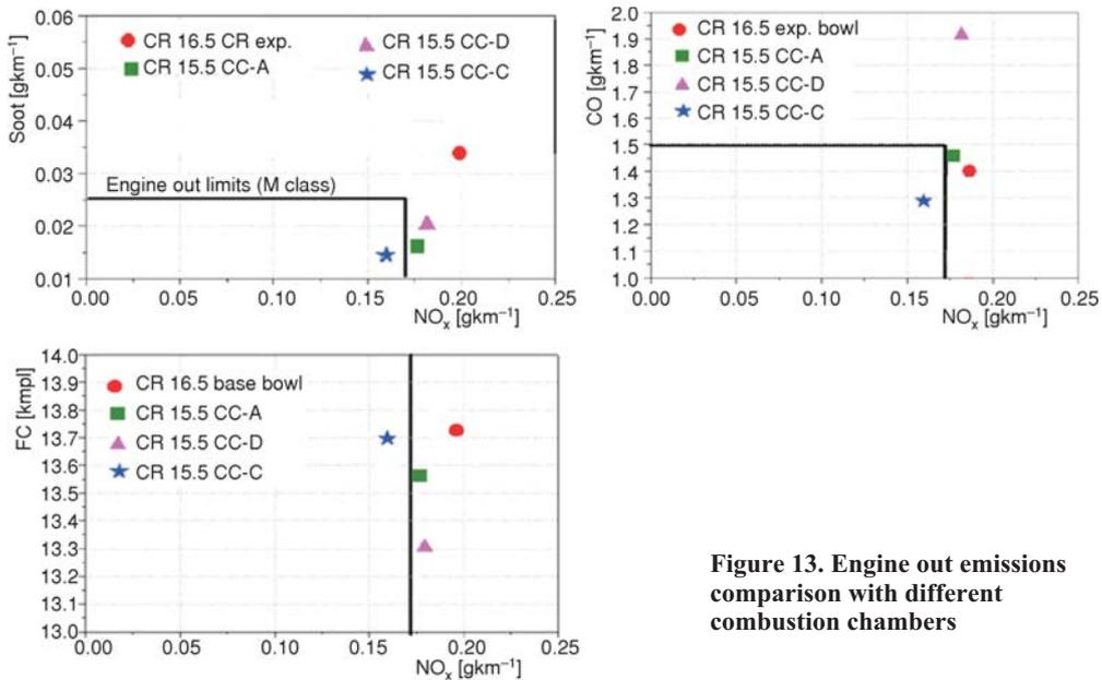
Figure 13. Engine out emissions comparison with different combustion chambers
