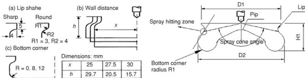
Figure 2. Critical parameters of combustion chamber design
