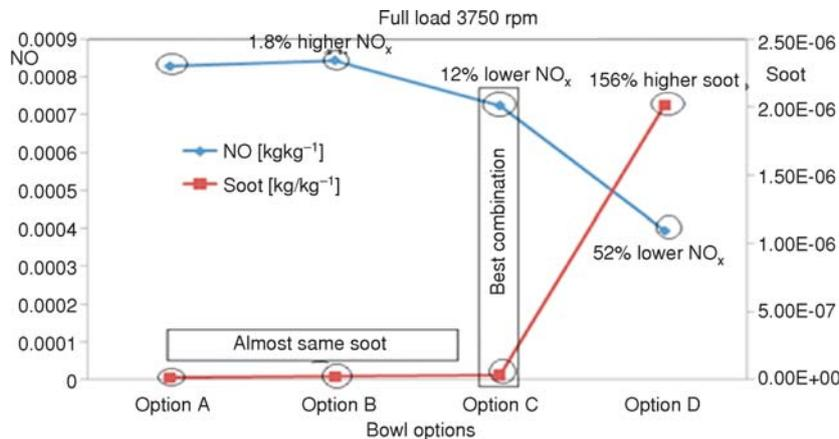
Figure 8. Cumulative NO comparisons and soot of different combustion chambers at 3750 rpm full load point
