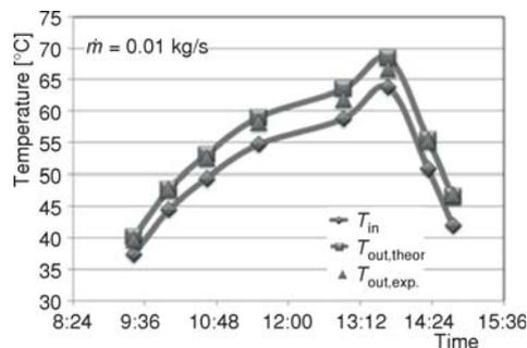
**Figure 5. Comparison between theoretical and experimental values of outlet water temperature at  $\dot{m} = 0.01$  kg/s****Table 3. Comparison between theoretical and experimental values of outlet water temperature at  $\dot{m} = 0.01$  kg/s**
