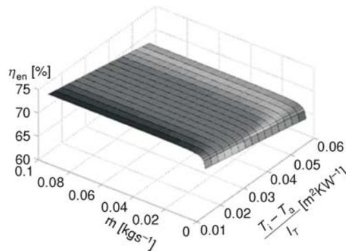
Figure 7. Energy efficiency vs. water mass flow rate and  $(T_{in} - T_a)/I_T$
