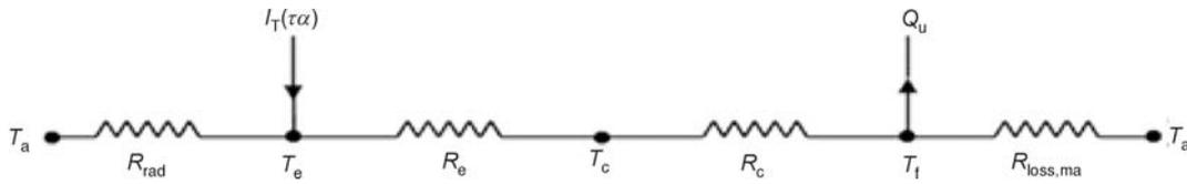
Figure 2. The electrical model for heat transfer in heat pipe evacuated collector
