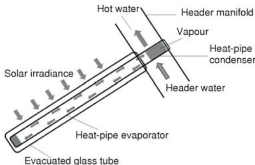
**Figure 1. Schematic view of the heat pipe evacuated solar collector**
