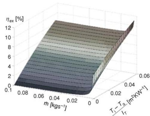
Figure 8. Exergy efficiency vs. water mass flow rate and  $(T_{in} - T_a)/I_T$
