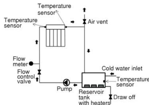
Figure 3. Schematic view of the investigated system
