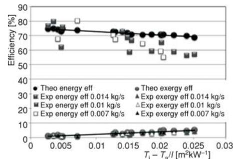
**Figure 6. Comparison between theoretical and experimental energy and exergy efficiencies**
