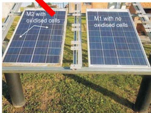
Figure 10. Oxidised cells on M2
