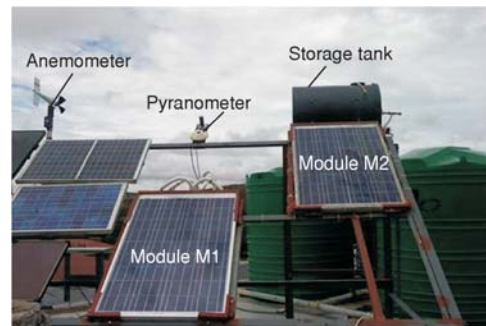
Figure 1. Naturally cooled (M1) and directly water cooled (M2) PV modules on a test rig
