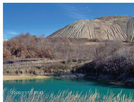
Figure 1. A photograph of the dump, formed of out of balance ore (top part), and the pond (lower part of the photo), formed by collecting the AMD.
