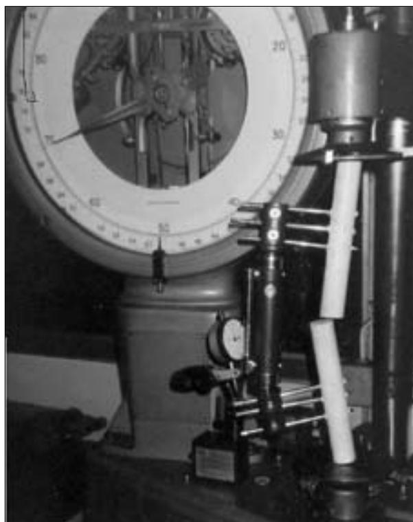
**Figure 2.** Physical model of juvidur – Ortofix fixator
