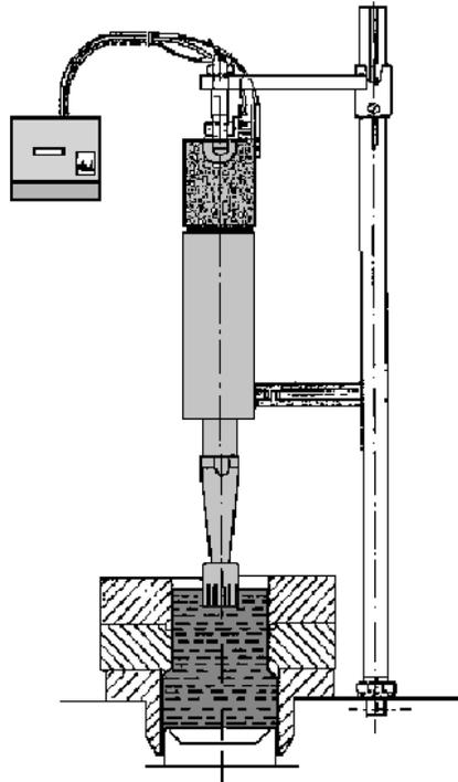
*Fig. 1. Ultrasonic head*
