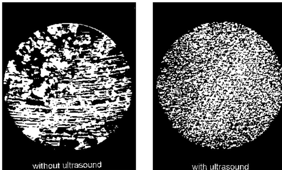
*Fig. 2. Aluminum structure without and with ultrasound*
