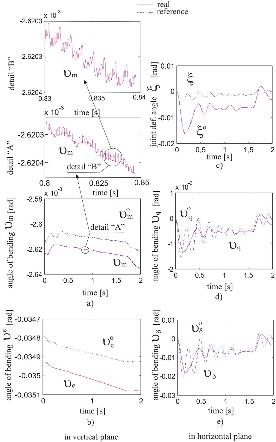
Figure 8: The elastic deformations.
