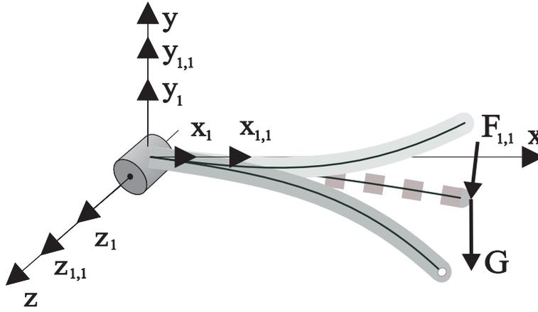
Figure 2: The motion of elastic body in case of gravity force presence.
