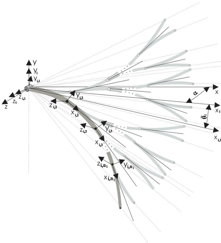
Figure 3: The possible positions of the elastic segment tip.
