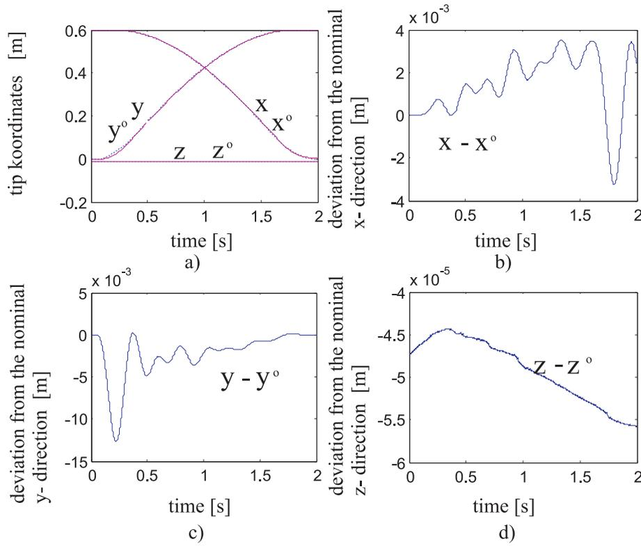
Figure 6: The tip coordinates and the position deviation from the reference level.
