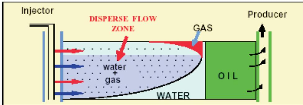
Figure 1: Schematic of the gas-water gravity segregation in far-wellbore region
