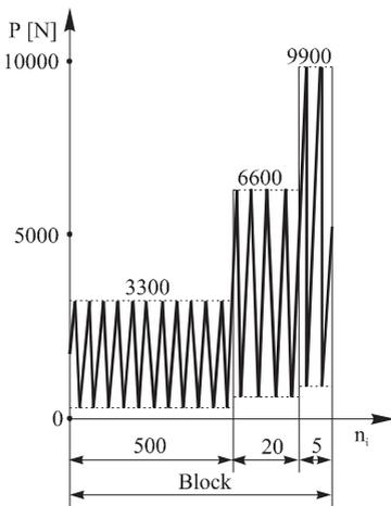
**Figure 6.** Load spectrum ( $R = 0.1$ )
