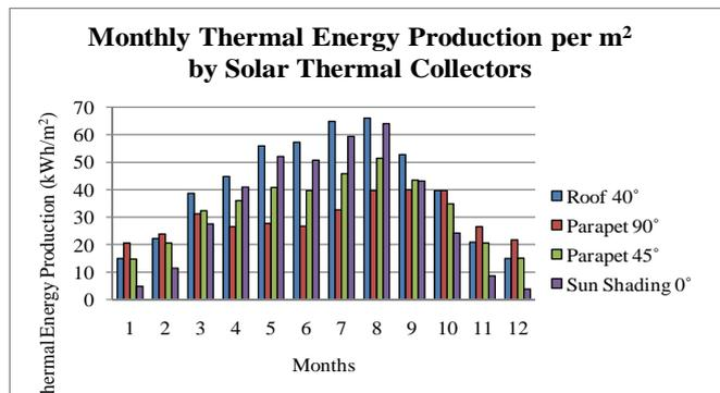
Figure 8: Monthly Thermal Energy Production per m<sup>2</sup> by Solar Thermal Collectors
