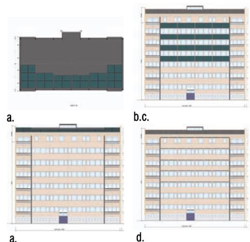
Figure 5: Analyzed design variants: a. I Design Variant: roof 40° (roof and facade layouts), b. II Design Variant: parapet 90°, c. III Design Variant: parapet 45°, d. IV Design Variant: sun shading 0°
