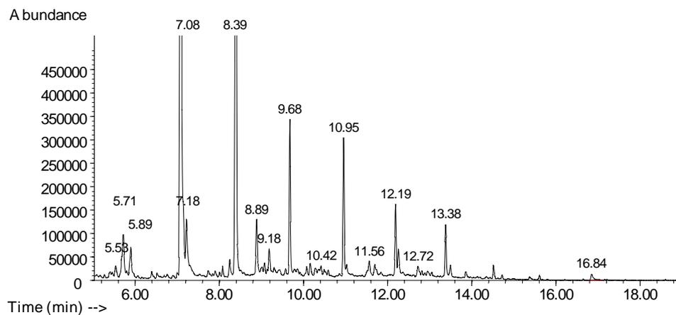
**Fig. 1.** GC-chromatogram of thyme *TE* obtained by liquid carbon dioxide
