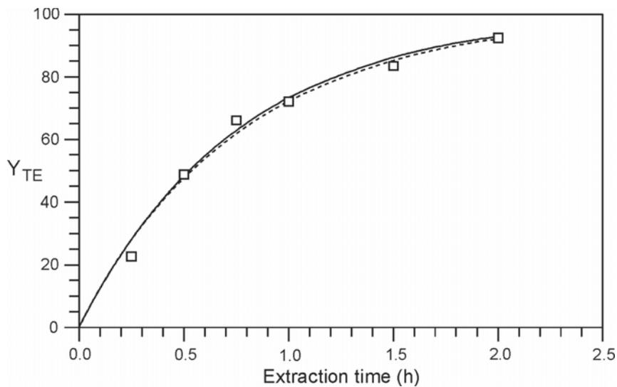
**Fig. 2.** Graphical presentation of Eq. [1] (solid line) and Eq. [2] (dashed line) and the experimental values ( $\sim$ ) of total extract ( $TE$ ) normalized extraction yield ( $Y_{TE}$ )
