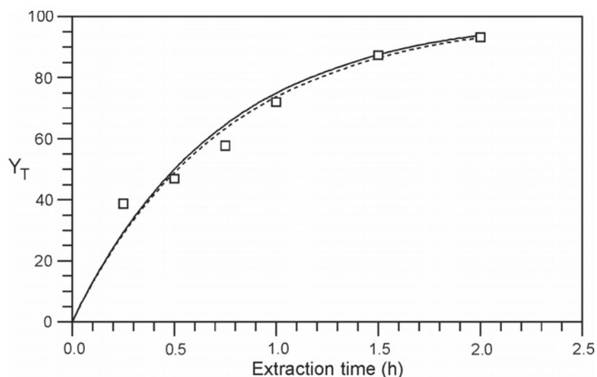
**Fig. 3.** Graphical presentation of Eq. [1] (solid line) and Eqs. [2] (dashed line) and the experimental values ( $\sim$ ) of thymol ( $T$ ) normalized extraction yield ( $Y_T$ )
