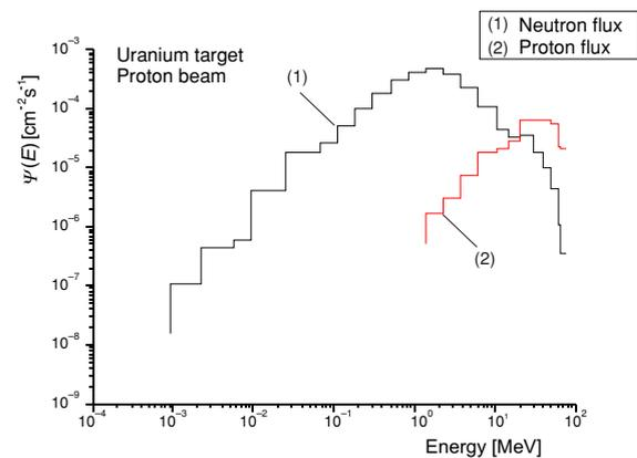
Figure 4. Particle flux escaping an uranium target – proton beam
