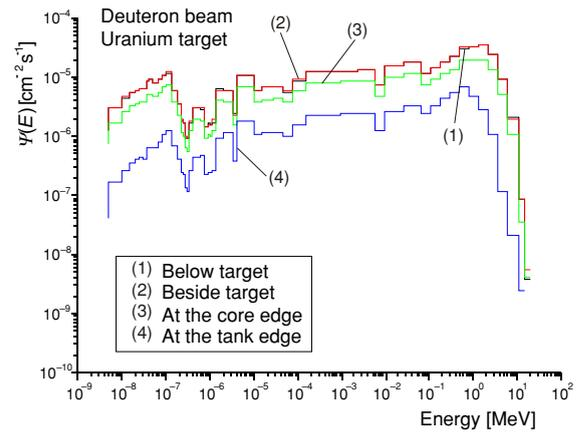
**Figure 7. Neutron flux in H5B ADSRF with an uranium target and a deuteron beam**
