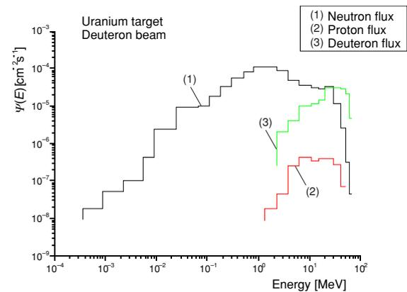
Figure 3. Particle flux escaping an uranium target – deuteron beam
