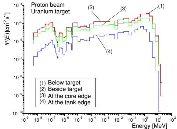
**Figure 8. Neutron flux (normalized) in H5B ADSRF with an uranium target and a proton beam****Table 6. Total neutron flux in cells for H5B ADSRF with an uranium target**
