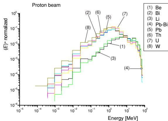
**Figure 6. Neutron flux (normalized) for different target materials – proton beam**
