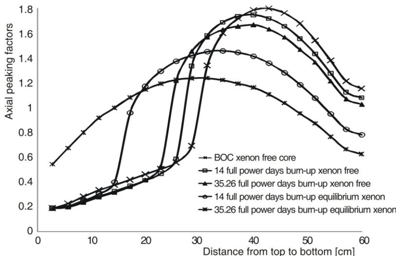
**Figure 4. Nuclear peaking factor (radial axial) along hot channel**
