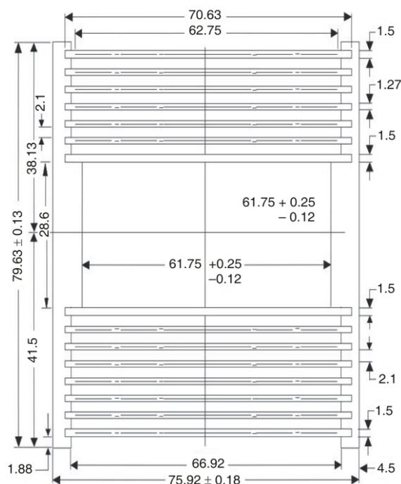
**Figure 3. LEU control fuel element cross-section**
