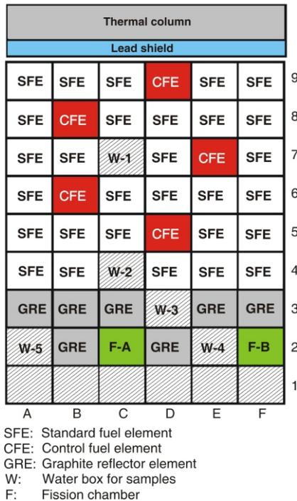
Figure 1. Core configuration
