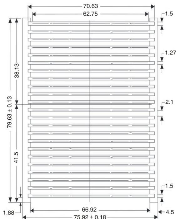
**Figure 2. LEU standard fuel element cross-section**
