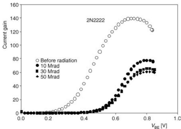
Figure 8. Plot of current gain  $\beta$  vs. base-emitter voltage  $V_{BE}$  with increasing dose for Si NPN BJT 2N2222 using Co-60
