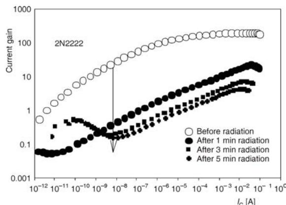
Figure 1. Plot of current gain  $\beta$  vs. collector current  $I_C$  with increasing radiation time for Si NPN BJT 2N2222 using PTS (neutron)
