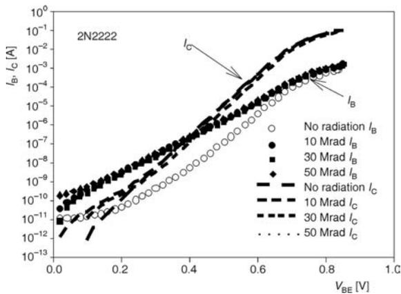
**Figure 12.** Plot of base current  $I_B$  and collector current  $I_C$  vs. base-emitter voltage  $V_{BE}$  irradiated with gamma radiation for Si NPN BJT 2N2222
