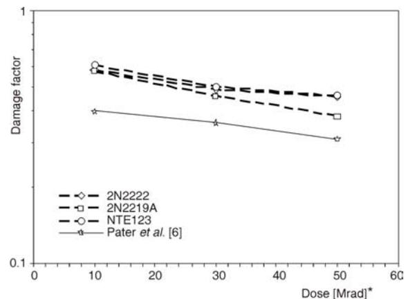
Figure 11. Plot of damage factor  $d_h$  vs. dose for all Si BJT at  $V_{BE} = 0.8$  V
