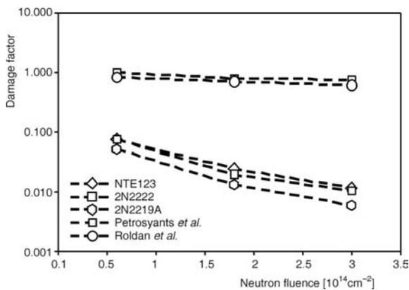
Figure 4. Plot of damage factor  $d_h$  vs. neutron fluence for all Si BJT measured at  $V_{BE} = 0.8$  V
