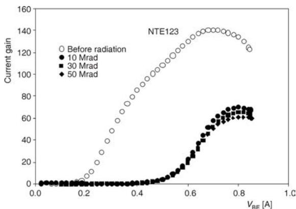
Figure 9. Plot of current gain  $\beta$  vs. base-emitter voltage  $V_{BE}$  with increasing dose for Si NPN BJT NTE123 using Co-60
