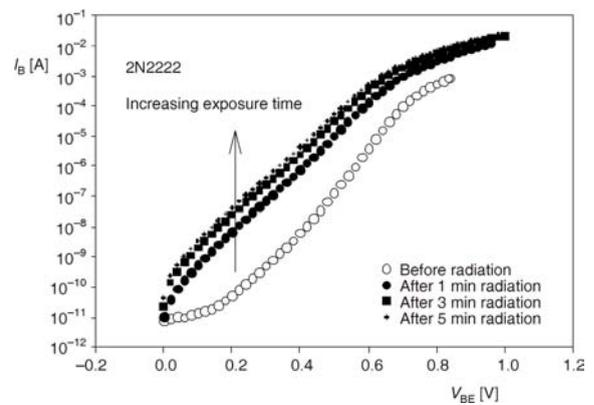
Figure 6. Plot of base current  $I_B$  vs. base-emitter voltage  $V_{BE}$  with increasing radiation time for Si NPN BJT NTE123 using PTS (neutron)
