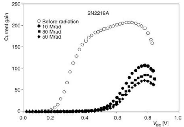
Figure 10. Plot of current gain  $\beta$  vs. base-emitter  $V_{BE}$  with increasing dose for Si NPN BJT 2N2219A using Co-60
