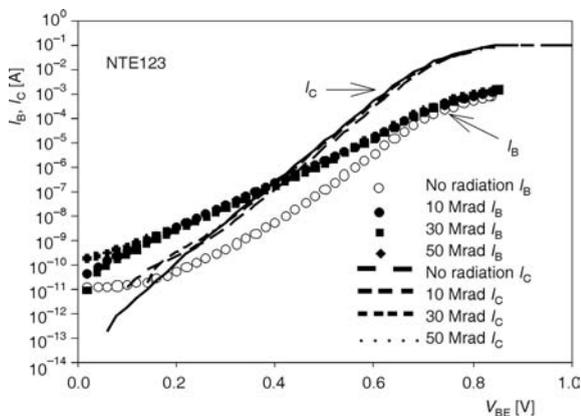
**Figure 13.** Plot of base current  $I_B$  and collector current  $I_C$  vs. base-emitter voltage  $V_{BE}$  irradiated with gamma radiation for Si NPN BJT NTE123
