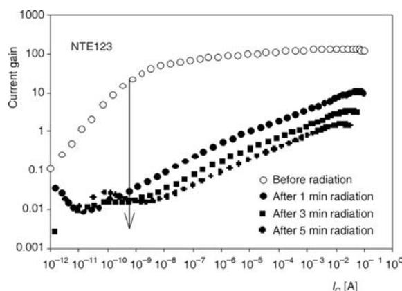
Figure 2. Plot of current gain  $\beta$  vs. collector current  $I_C$  with increasing radiation time for Si NPN BJT NTE123 using PTS (neutron)
