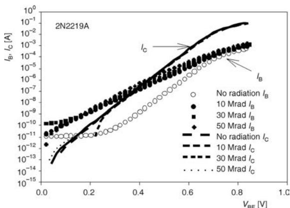
**Figure 14.** Plot of base current  $I_B$  and collector current  $I_C$  vs. base-emitter voltage  $V_{BE}$  irradiated with gamma radiation for Si NPN BJT 2N2219A
