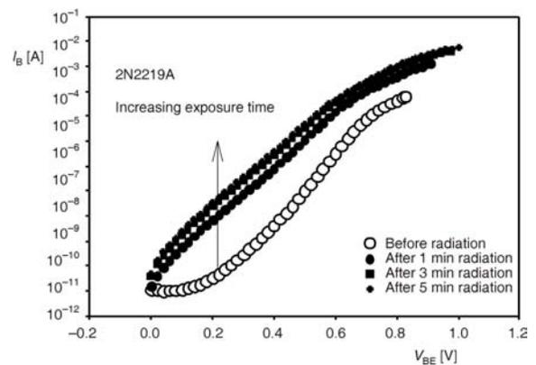
Figure 7. Plot of base current  $I_B$  vs. base-emitter voltage  $V_{BE}$  with increasing radiation time for Si NPN BJT 2N2219A using PTS (neutron)
