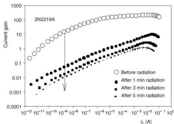
Figure 3. Plot of current gain  $\beta$  vs. collector current  $I_C$  with increasing radiation time for Si NPN BJT 2N2219A using PTS (neutron)
