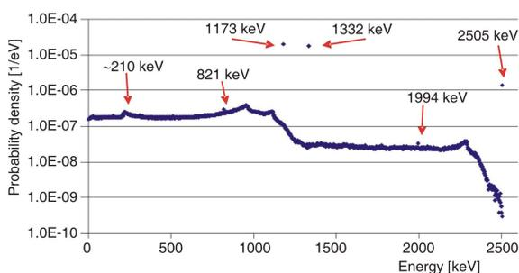
**Figure 1. Simulation spectrum of a  $^{60}\text{Co}$  point source on the XtRa detector endcap**
