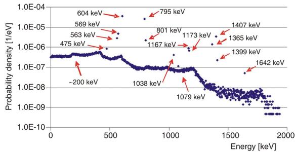
**Figure 2. Simulation spectrum of a  $^{134}\text{Cs}$  point source on the XtRa detector endcap**
