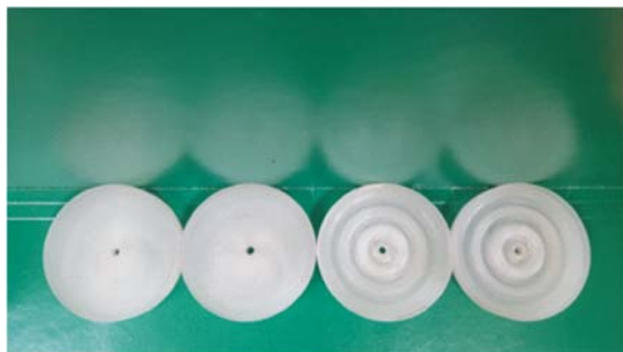
Figure 4. Spacers/holders for the central electrode (type I and II)
