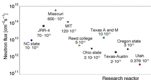
**Figure 1. Thermal neutron flux for irradiation ports in research reactors with NAA facilities. (Neutron flux data taken from the individual organizations' web sites)**
