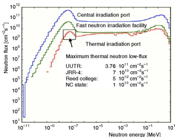
Figure 2. Neutron flux profile as a function of neutron energy in the UUTR irradiation ports (calculated with MCNP6); the UUTR has a maximum thermal neutron flux of  $3.76 \cdot 10^{11} \text{ cm}^{-2}\text{s}^{-1}$  as shown in fig. 1
