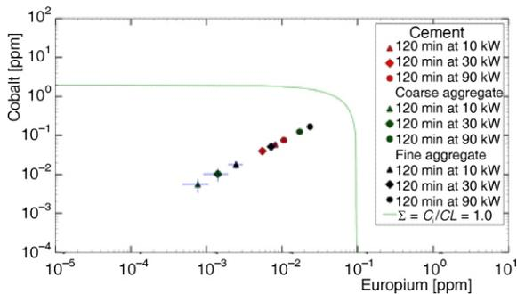
**Figure 3.** Calculated trace concentrations of Co and Eu in white cement, coarse, and fine aggregates using standard reference material 1333c Coal fly ash for white cement and 2710a Montana soil for coarse and fine aggregates. Samples enclosed in green represent samples that fall below IAEA established clearance levels for LLW
