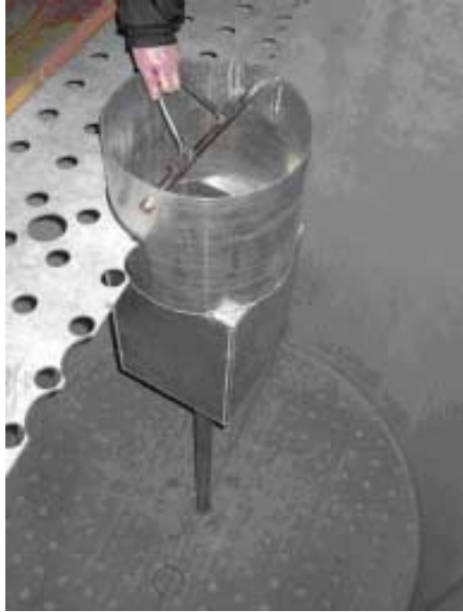
Fig. 3 - Aluminum vessel of the INC at the position inside the RB reactor tank.
