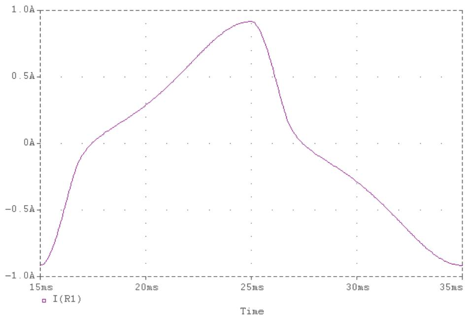
**Fig. 2** – Switching transients simulation -  $\beta = 0$ .
