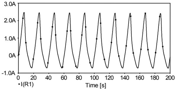
**Fig. 6** – Switching transients simulation -  $\beta = \pi/4$  .
