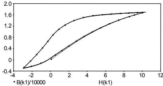
**Fig. 7** – Switching transients simulation of  $B(H)$  loop –  $\beta = \pi/4$ .
