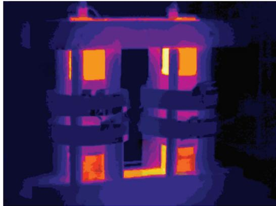
**Fig. 8** – The temperature distribution in ferrite core.
