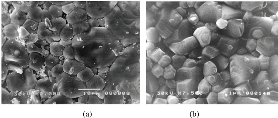
**Fig. 2** – SEM images of (a) 0.5 wt % and (b) 1 wt % Ho/BaTiO<sub>3</sub> sintered at 1380°C.
