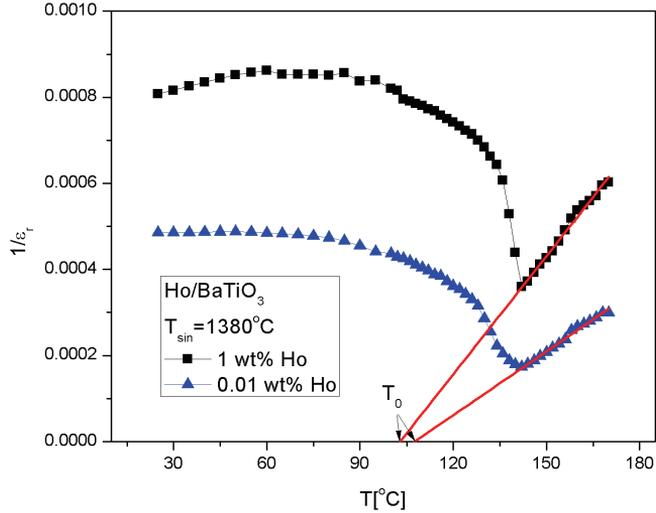
**Fig. 9** – Temperature dependence of reciprocal value of  $\epsilon_r$  for 0.01 wt % and 1 wt % of Ho doped BaTiO<sub>3</sub>.
