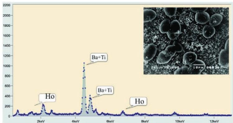
**Fig. 3** – SEM/EDS image of 0.5 wt % Ho/BaTiO<sub>3</sub>.
