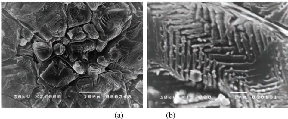
**Fig. 5** – Domain structure of 0.01 wt % Ho/BaTiO<sub>3</sub> sintered at 1380°C
