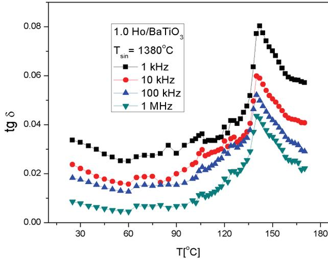
**Fig. 8** – Temperature dependence of dissipation losses of doped BaTiO<sub>3</sub> ceramics for different frequencies ( $c = 1$  wt % of Ho).
