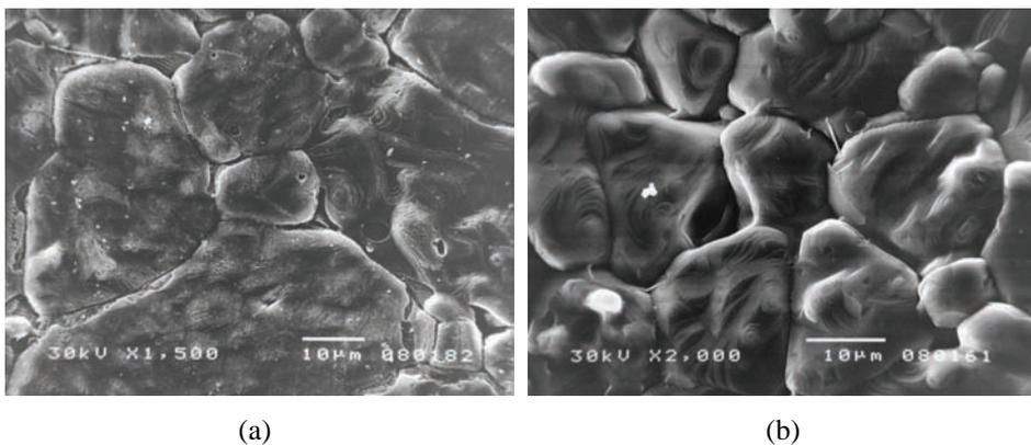
**Fig. 1** – SEM images of (a) 0.01 wt % and (b) 0.1 wt % Ho/BaTiO<sub>3</sub> sintered at 1380°C.
