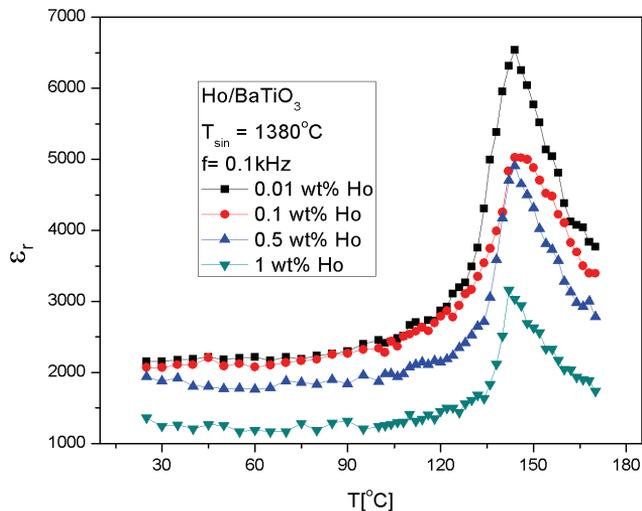
**Fig. 7** – Temperature dependence of dielectric relative permittivity of doped BaTiO<sub>3</sub> ceramics for different concentration of Ho at  $f = 0.1$  kHz.
