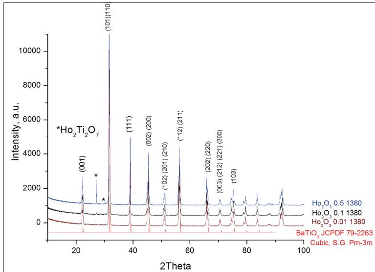
**Fig. 4** – X-ray diffraction pattern for Ho/BaTiO<sub>3</sub> samples.
