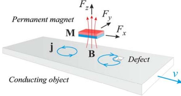
**Fig 1** – Basic principle of LET. The conductive specimen moves with velocity  $v$  relative to a permanent magnet. The interaction between the primary magnetic field and the induced eddy currents in the specimen results in Lorentz force components  $F_x$ ,  $F_y$  and  $F_z$  exerted on the permanent magnet.
