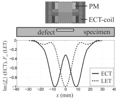
**Fig. 4** – Normalized defect response signals of LET and ECT.
