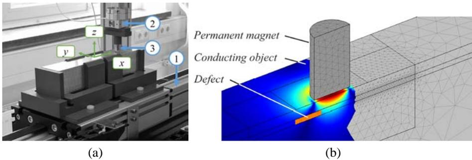
**Fig. 3** – (a) Experimental setup with linear drive (1), 3D force sensor (2), permanent magnet (3) and 2D linear stage (not shown); (b) 3D FEM model used for LET simulations.
