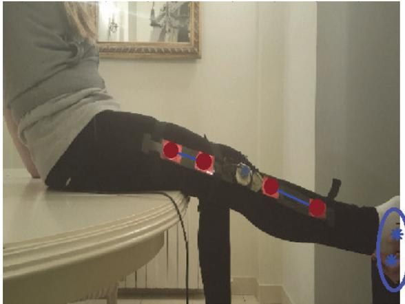
**Fig. 10** – False detected markers due to the inadequate background are shown with asterisks on foot.
