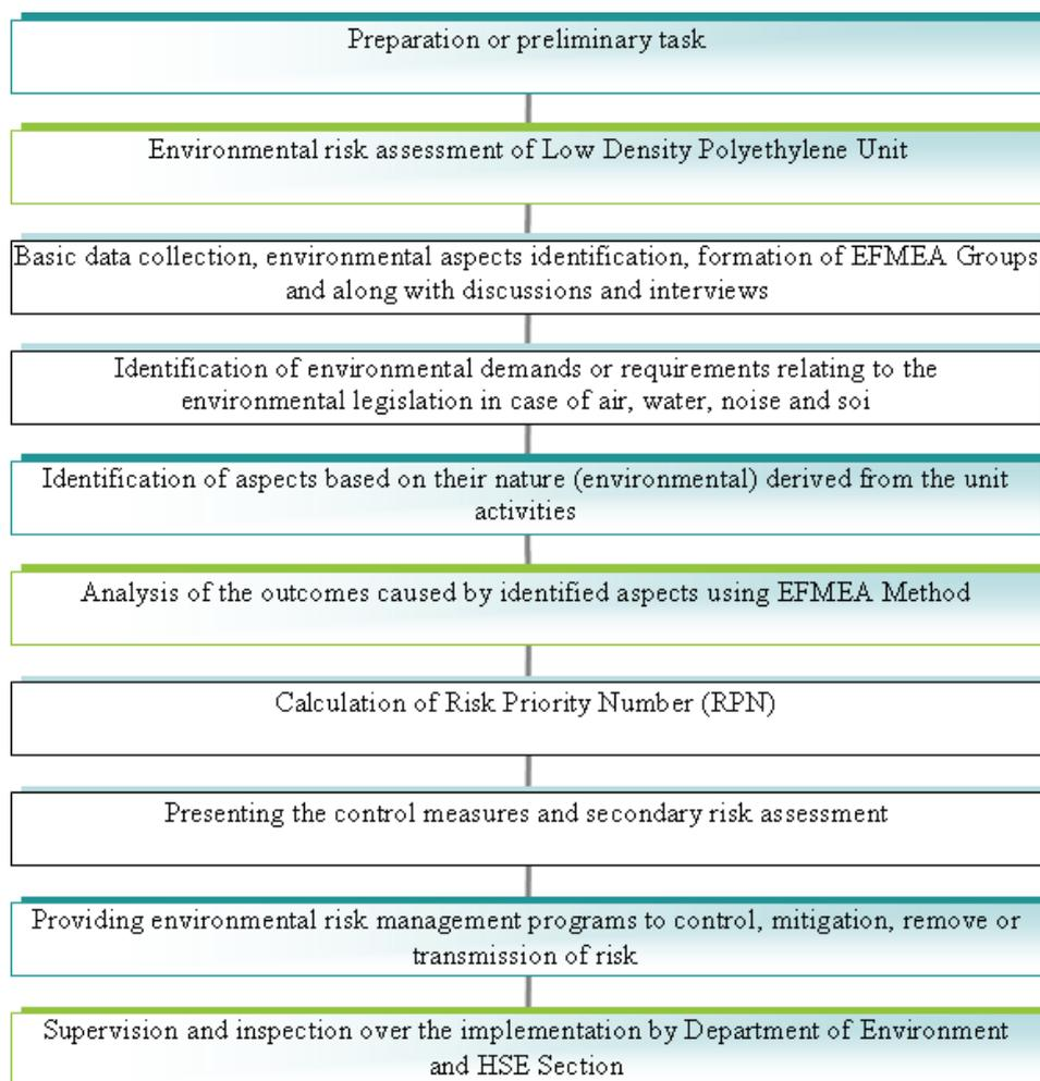
Figure 2. Workflow process in Low Density Polyethylene Unit.
