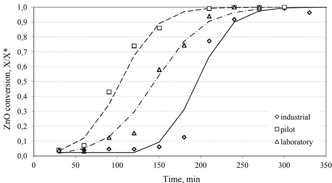
Figure 4. ZnO Conversion vs. time graph of the experiments to observe the effect of scale-up (temperature 85 °C, seed amount 1.5%, initial reactants ratio ( $H_3BO_3$ :ZnO ratio of 5:1), and average particle size of zinc oxide particles of <math><1 \mu m</math> were constant). Curves denote the logistic model.
