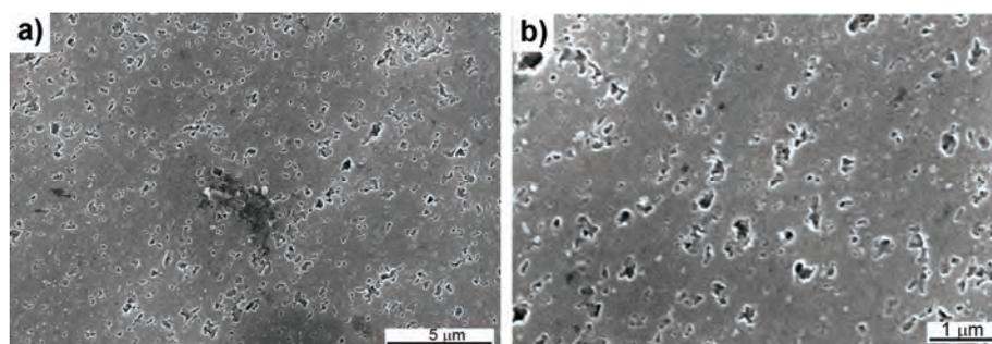
Figure 3. SEM microphotographs of the tested aluminum alloy after two-step aging.
