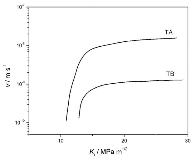
Figure 5.  $v$ - $K_I$  dependence for the tested aluminum alloy in TA and TB state.
