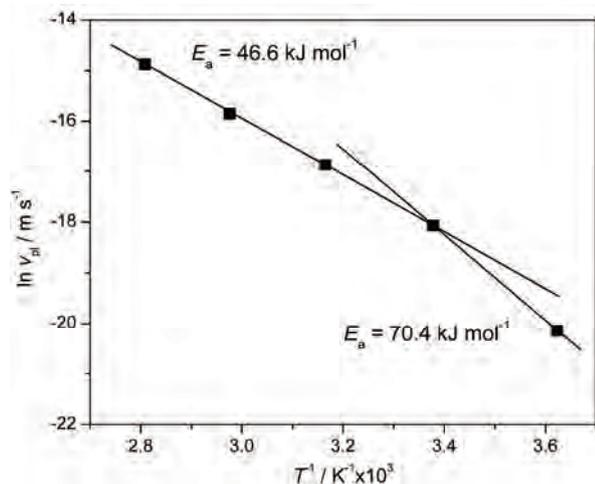
Figure 6. Temperature dependence of  $v_{pi}$  during SCC testing (TA state).
