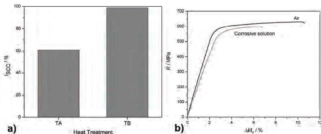
Figure 4. a)  $I_{SCC}$  values for the tested aluminum alloy in TA and TB state; b) Experimental stress - strain curve for the alloy in TA state.
