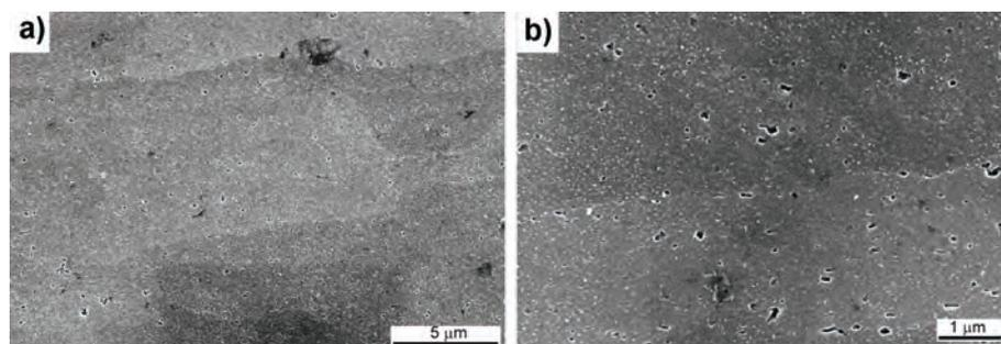
Figure 2. SEM microphotographs of the tested aluminum alloy after one-step aging.
