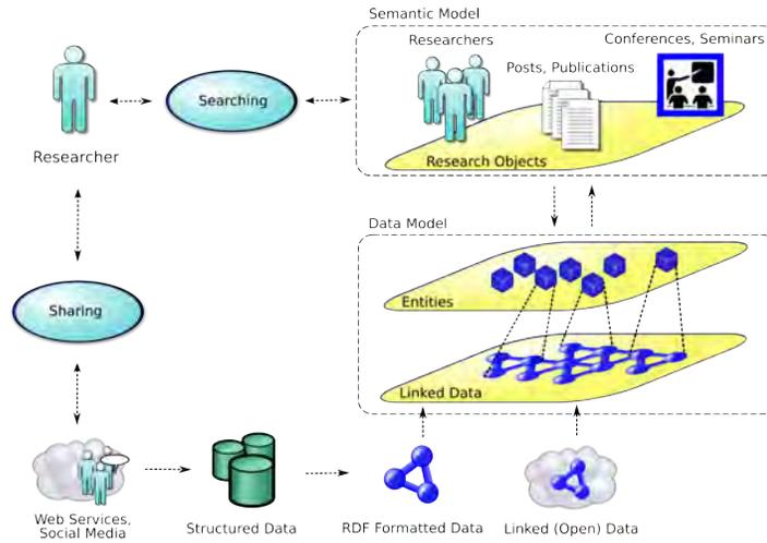
**Fig. 1.** The information researchers share via the Web services of research collaboration tools and social media is structured and transformed to RDF and interlinked with Linked Open Data. The resulting entities in the data model form the base for the semantic model. This process is outlined in Section 3.1. When researchers search, they interact indirectly with the semantic model which we detail in Section 3.2.
